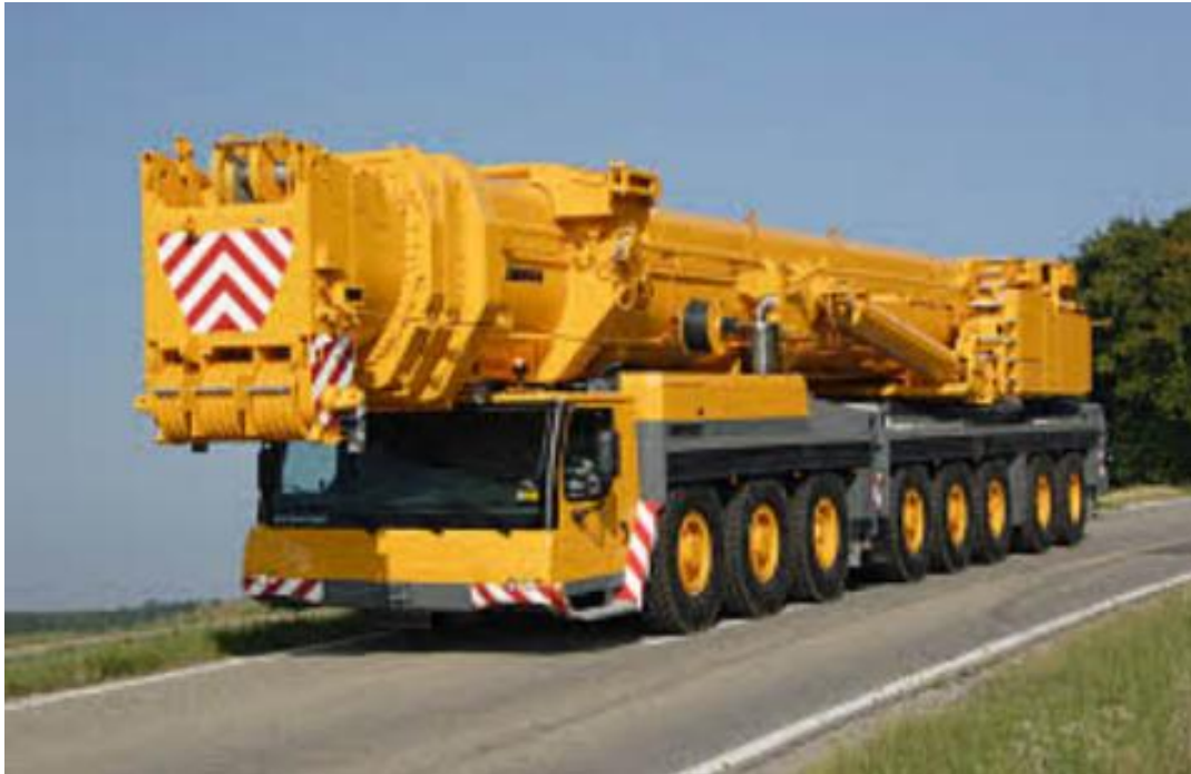
Plate 4.6: Crane for wind turbine erection 2
